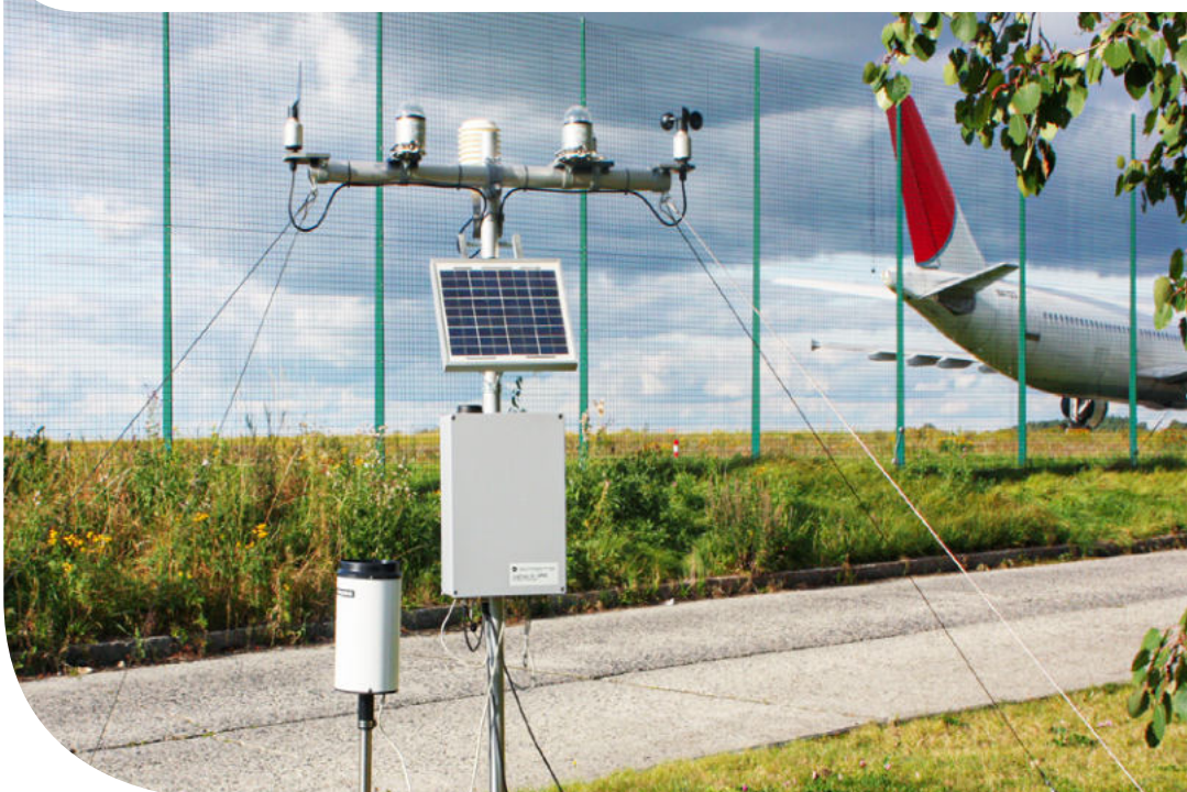
Meteorological measuring stations
