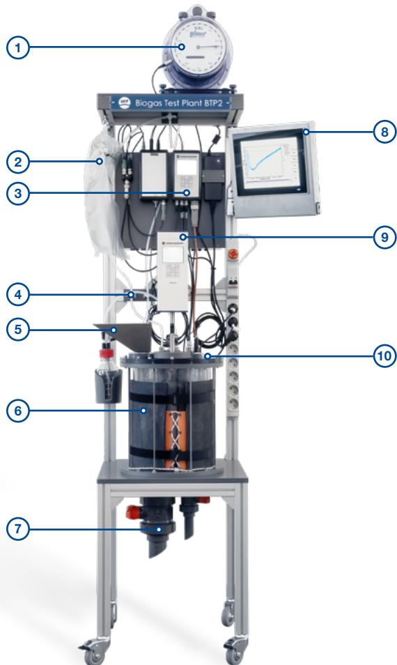
The biogas pilot plant BTP2 is the base system for substrate testing and gas potential tests and further research activities. This system is also ideally suited for product development (enzymes, nutrients) or for process optimization.
