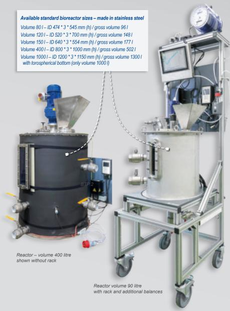
Standardized and customized bioreactors lab and pilot test facilities for biogas research, product development (enzymes, nutrients), process optimization and biotechnology application (research and piloting).
