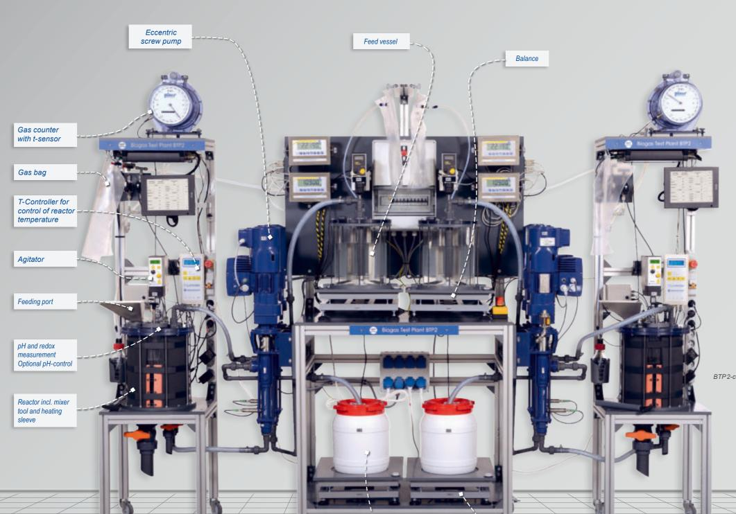
The individual BTP modules can also be equipped with eccentric screw pumps.
