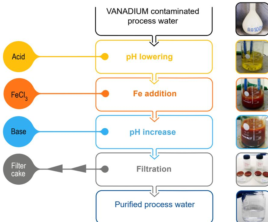
Figure 6: Block diagram of vanadium removal
