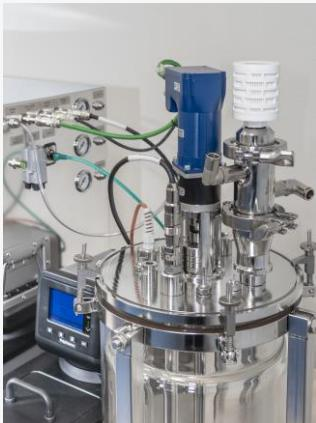
Interface for two **mixer units** incl. speed control
