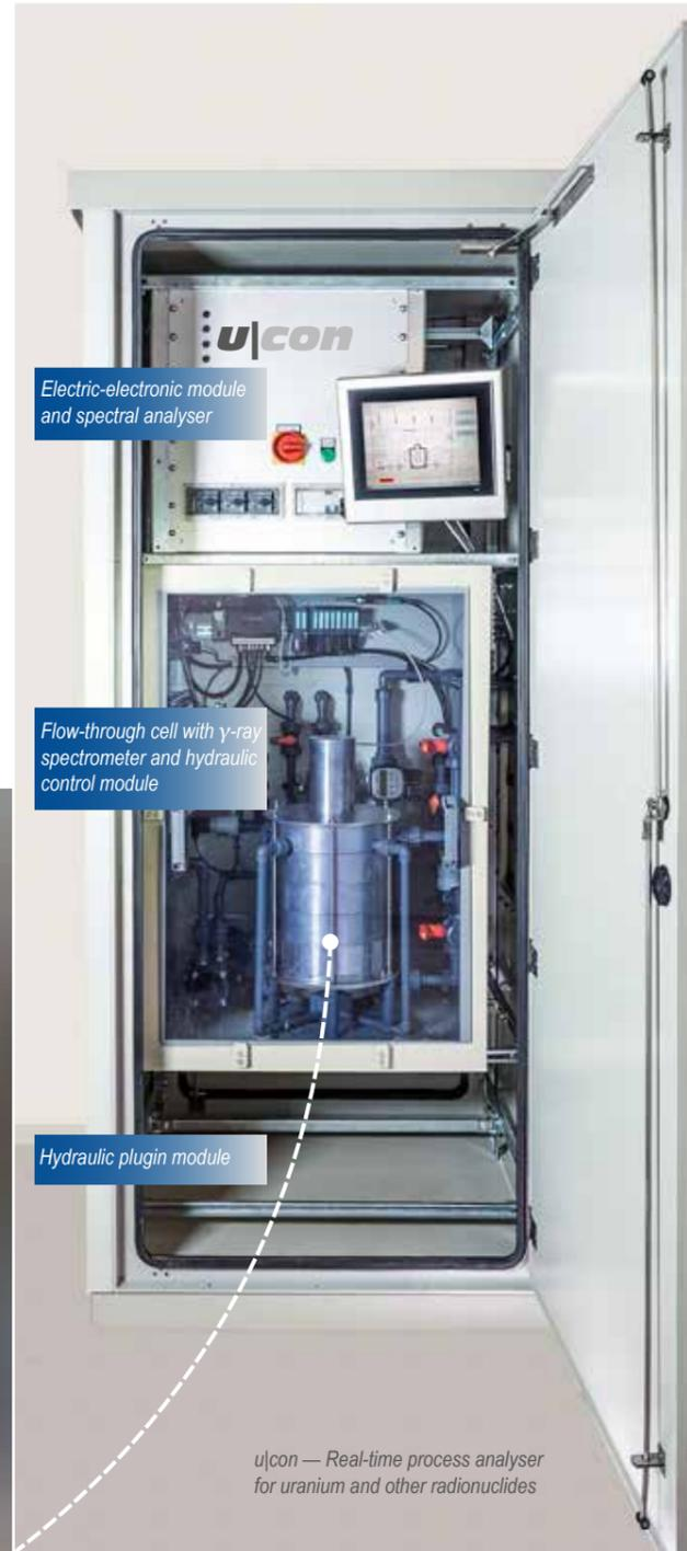
u|con — Real-time process analyser for uranium and other radionuclides
